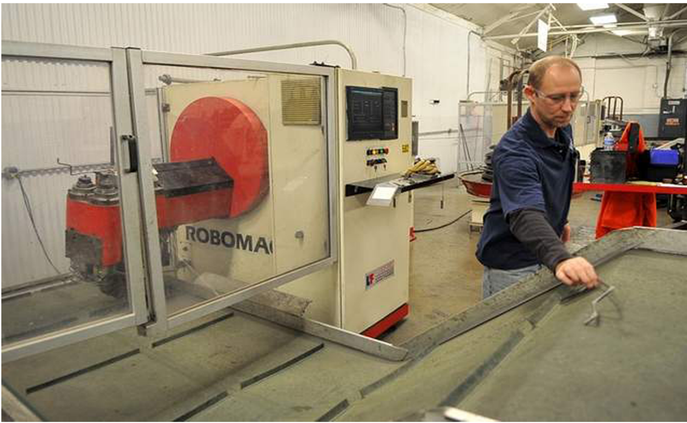
Joe Munyan picks up a belt guide for a riding lawn mower Friday to check the bends being made by the machine he runs at Mid West Fabrications Co. in Amanda. MATTHEW BERRY/EAGLE-GAZETTE
